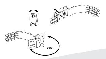
Fixed lateral supports are available for situations when a swing-away lateral is not required. Fixed lateral supports consist of shell bracket, pad bracket and pad.
